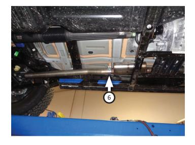
12. Place clamp (6) onto rear inlet pipe (4), then connect it to front inlet pipe. Insert wire hanger into isolator then tighten clamp just enough to allow for adjustment.
