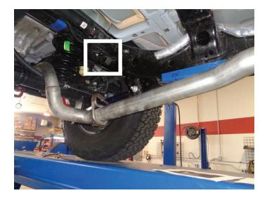
8. Remove bolt on clamp at resonator inlet then remove assembly from vehicle. Retain clamp for later re-use.
