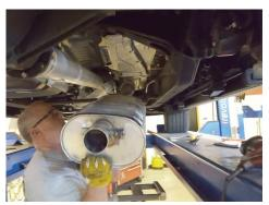
10. Release tab and remove clamp from muffler assembly. Retain for later use.
