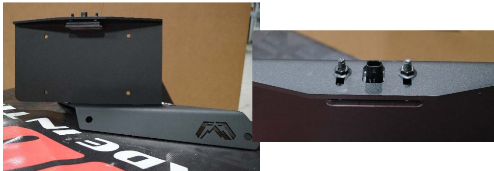
Figure 3a & 3b. Inserting the OEM license plate light into the M4550 license plate bracket.
