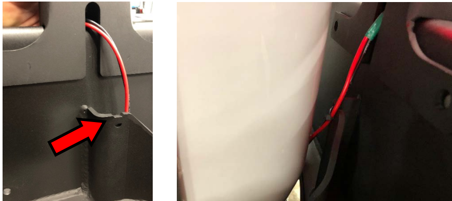
Figure 9a & 9b. Wiring connections for M4550 bracket installation.
