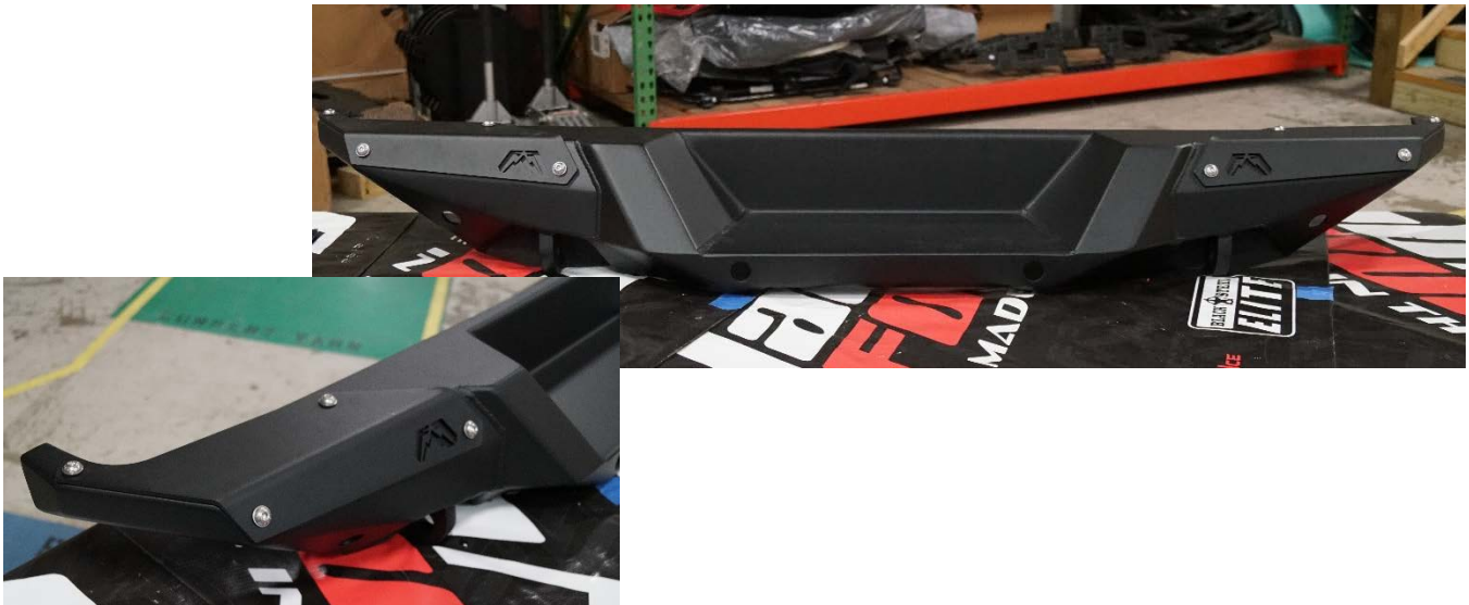
Figure 1a & 1b. Driver side cover plate on Y1851 bumper.
